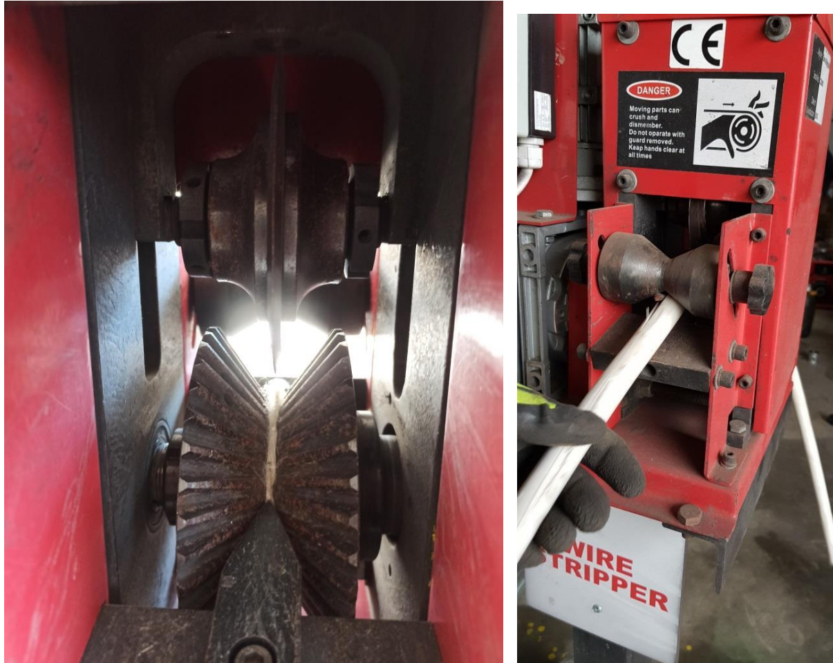
Figure 3.9: Rotating blade and wire stripping
