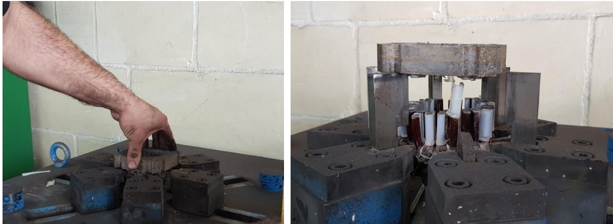
Figure 3.22: Extracted windings and steel component
