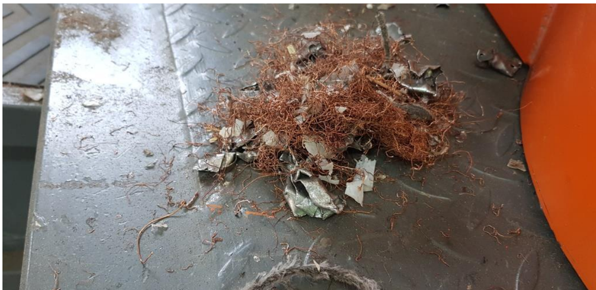
Figure 3.14: Mixed ferrous and non-ferrous metals from motor crusher
