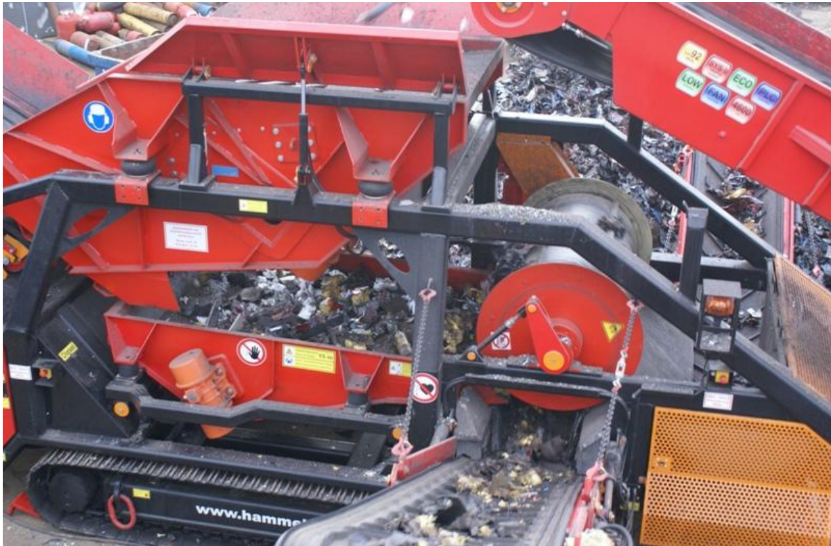
Figure 3.10: Sorting system, including magnetic drum
