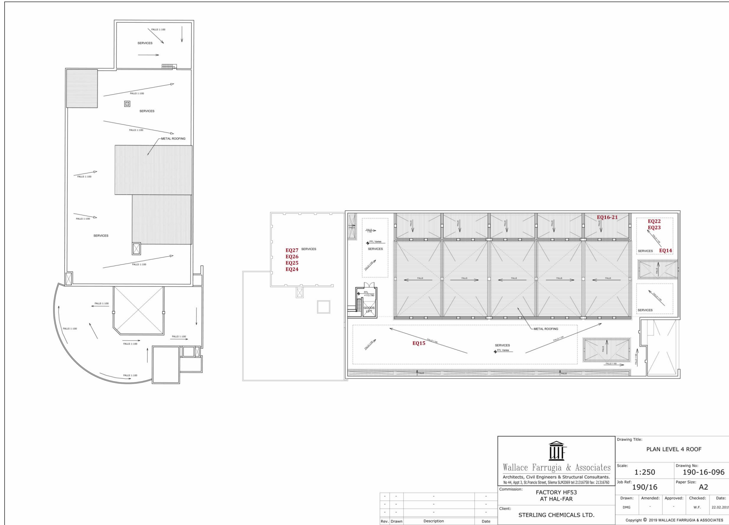
Figure 3.14: Location of refrigerant-containing equipment
