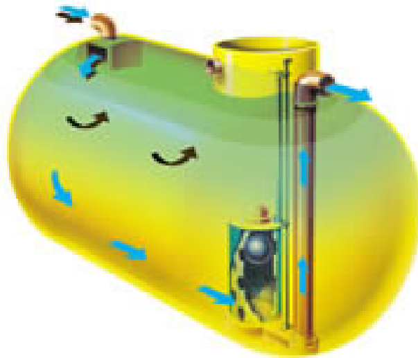
Figure 1.2: Diagram of a typical Fuel Separator
