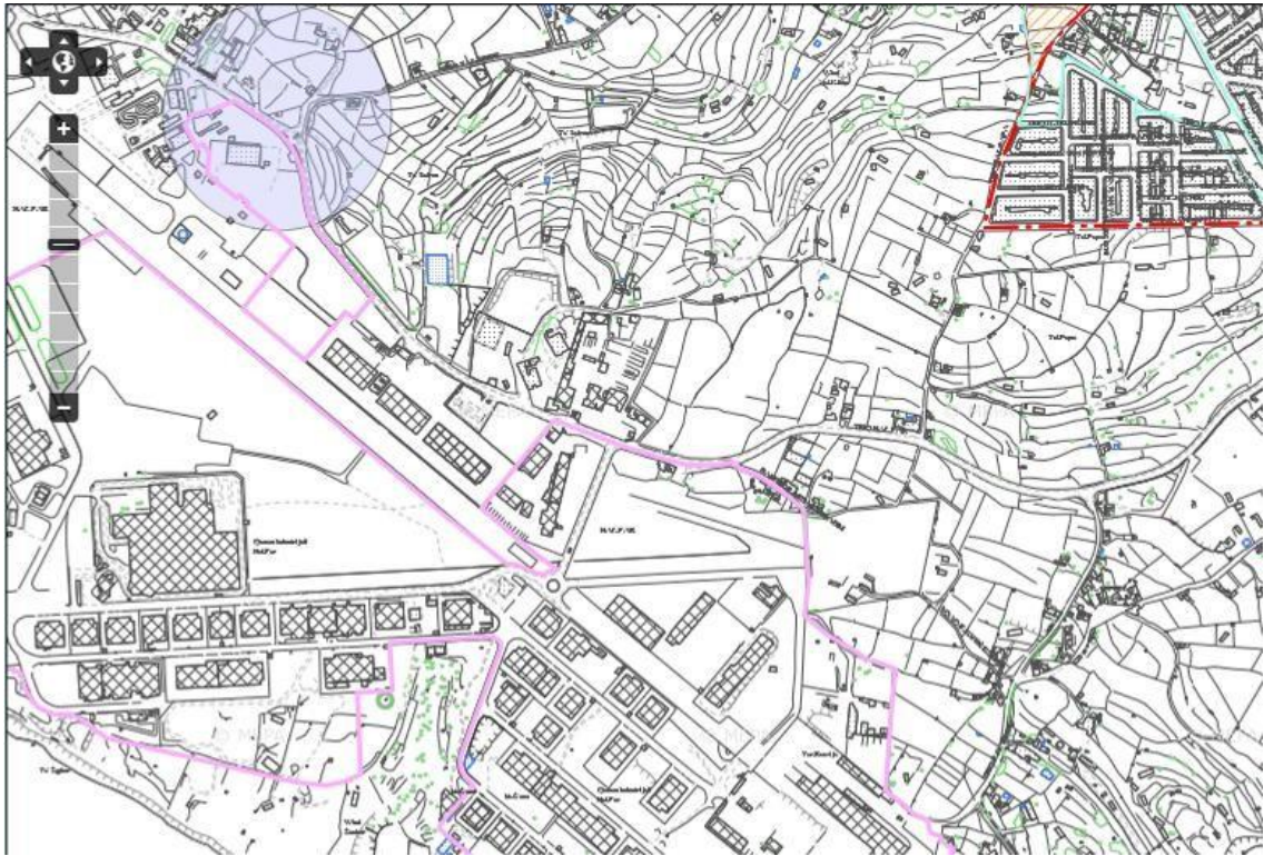
Figure 11: MEPA Mapserver map showing the closest WSC borehole surrounded by a 300m safe guard zone (Grey circle) at Hal Far Barracks
