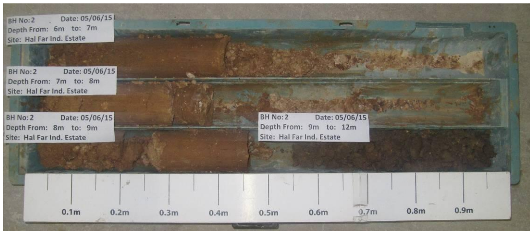
Plate 5: Photograph showing rock core samples recovered from BH2 run No.7 to run No.9 (For scale core tray is 100cm long)
