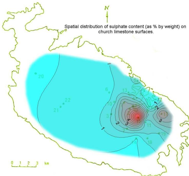
Figure 7 The distribution of degree of sulfation of church limestone surfaces (Vella et al., 1996)
