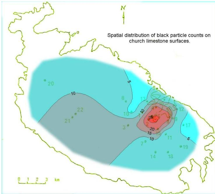
Figure 6: The distribution of black particles in church limestone surfaces (Vella et al., 1996)
