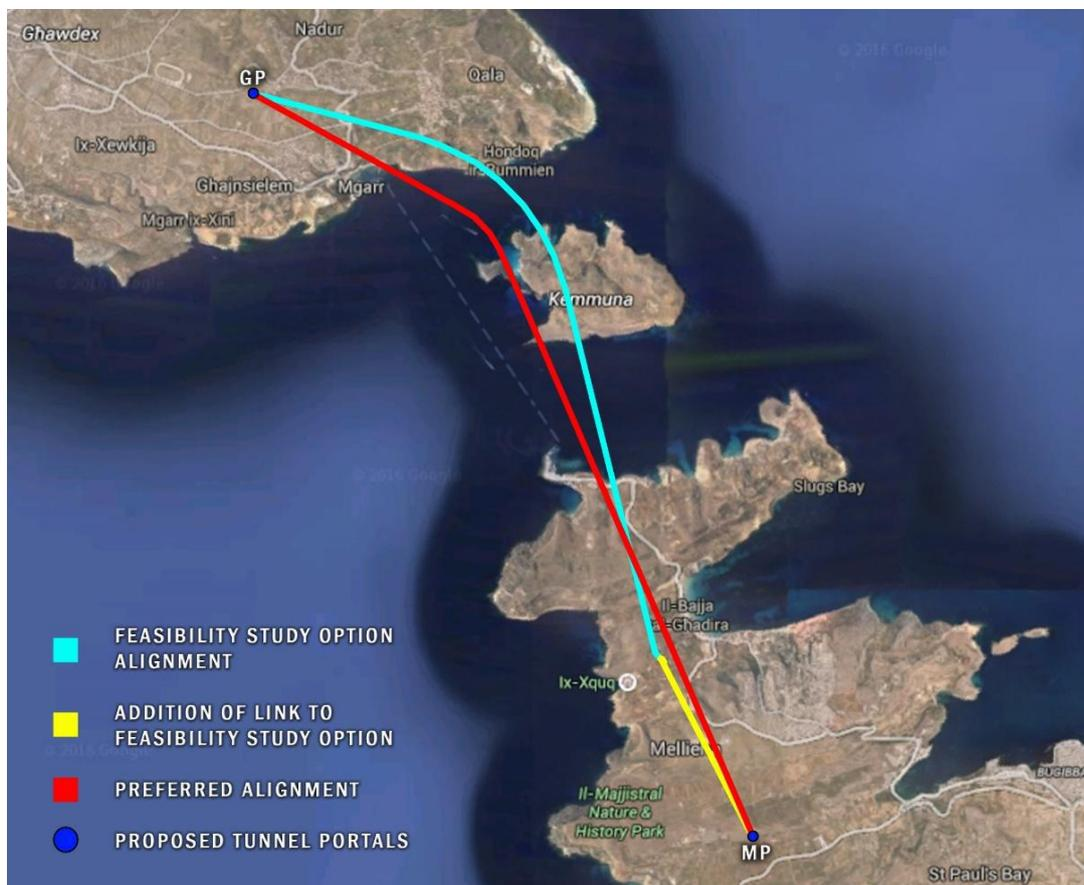
Figure 2 – Proposed tunnel alignment
