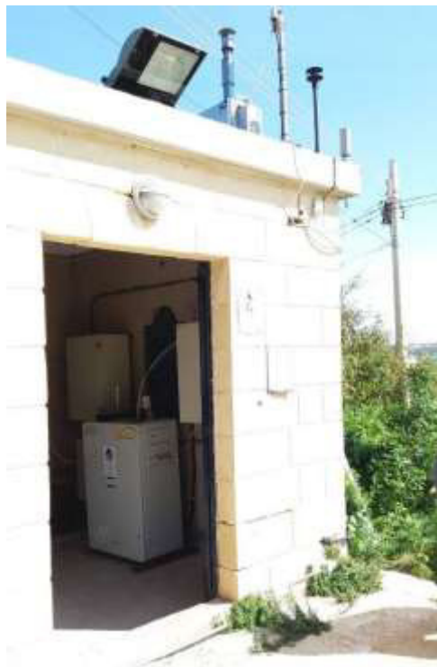
Figure 2. Photo showing the NO x and weather monitoring equipment installed on site.
