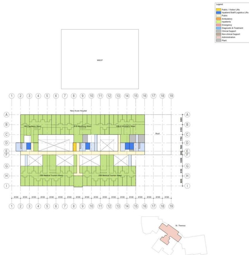
Figure 5: Level +2 plan (Source: PDS)
