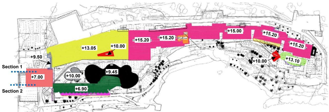
Figure 1-1 – proposed excavation plan (levels are relative to mean sea level)
