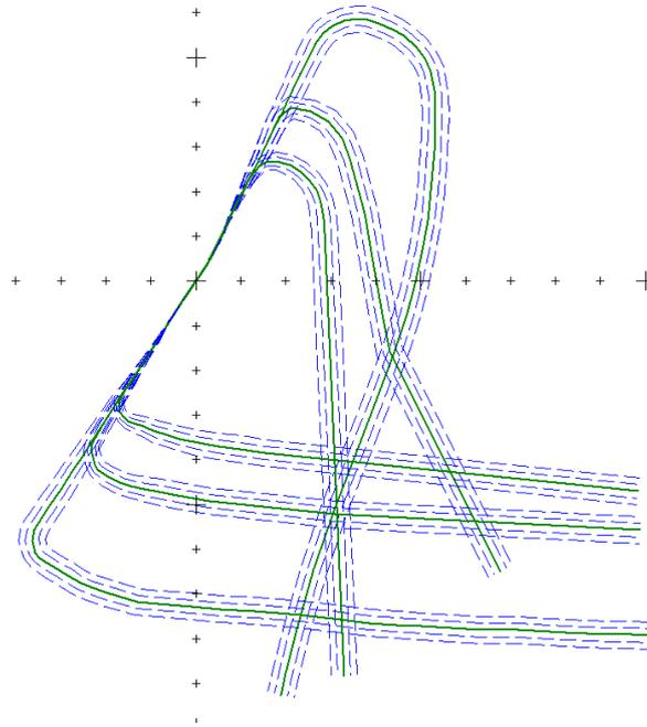
**Figure 8.1:** Modelled mean flight tracks and dispersion
