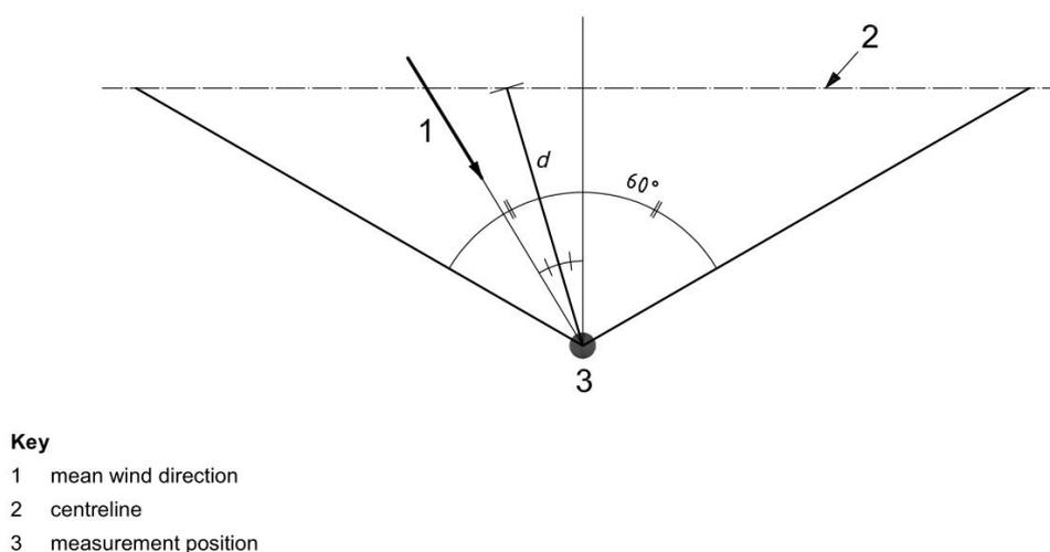
**Figure 12.7:** Favourable propagation conditions from a road and the effective source-receiver distance,  $d$
