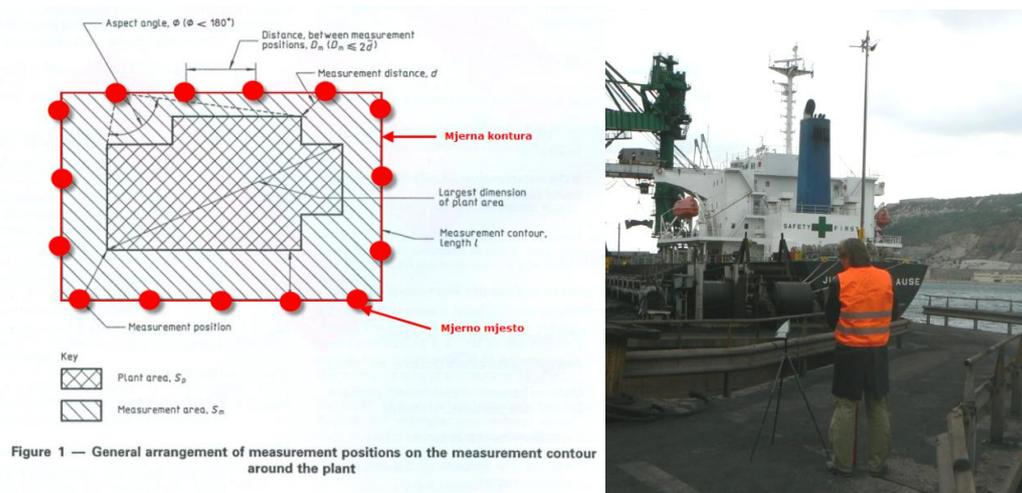
**Figure 12.6:** Graphical determination of the measurement contour (red line), measurement points (red points) and photo during measurements according to ISO 8297
