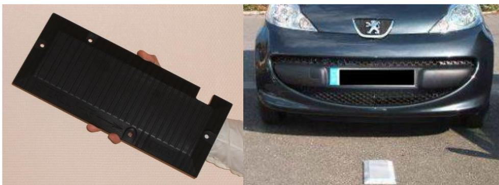
**Figure 12.1:** Portable traffic analyser
