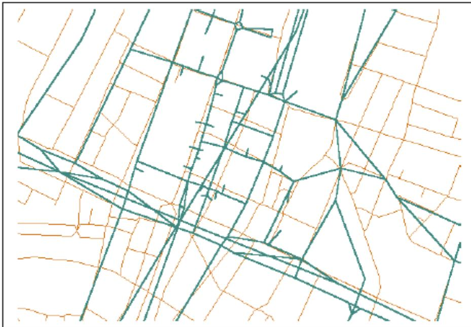
**Figure 8.2:** An example of an accurate digital road network model (brown) and an inaccurate road traffic network model (green). (After WG-AEN GPG v2 p19.)
