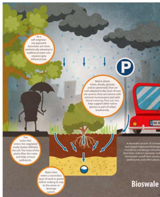
Figure 2: Design of possible implementation of a bioswale 'rain garden' at the identified location
