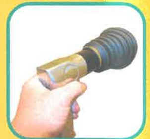
Pneumatic drill to pierce the shock absorber
