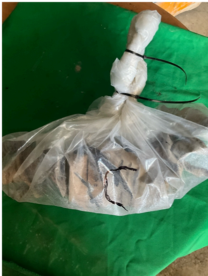
7. An image of a Type C Catalytic Converter contained within a heavy-duty polythene bag. The polythene bag has been secured by swan necking its opening and the application of 2 cable ties. This process is standard with all such units on arrival at the Hal Far site from the suppliers.
