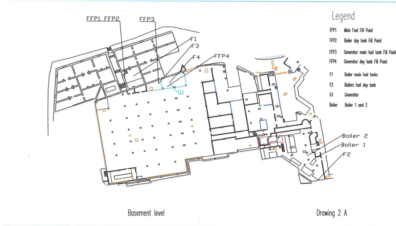
Fig.S.1.2a: Site layout of the permitted installation to undertake the operations specified in condition 1.1.1, showing the location of combustion plants, fuel storage areas and fuel fill points. The point locations are indicative and shall not be used for interpretation purposes.
