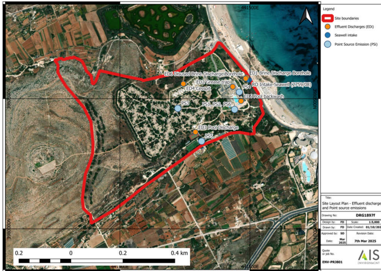
Fig S1.2: Site layout of the permitted installation to undertake the activities specified in condition 1.1.1, showing effluent discharge points, cesspit and emissions to air. The point locations are indicative and shall not be used for interpretation purposes.
