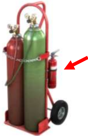
Image 1 – Oxy-acetylene set with fire extinguisher
