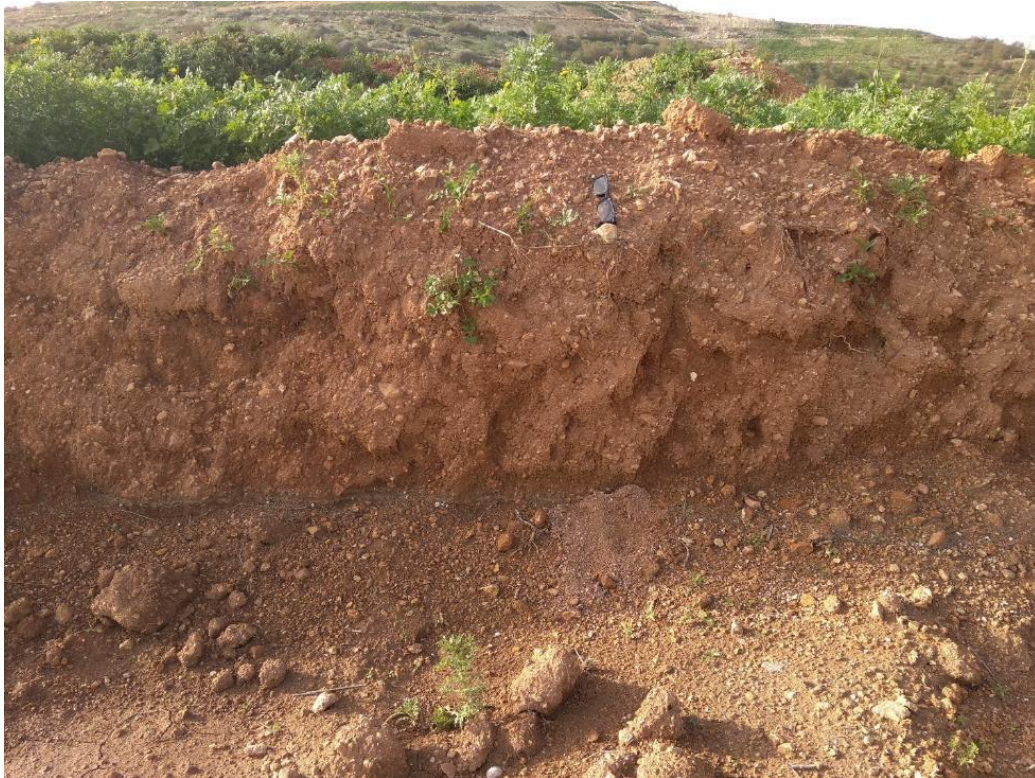
Figure 40: Photograph of a typical soil profile at the OPP site about 0.4m thick
