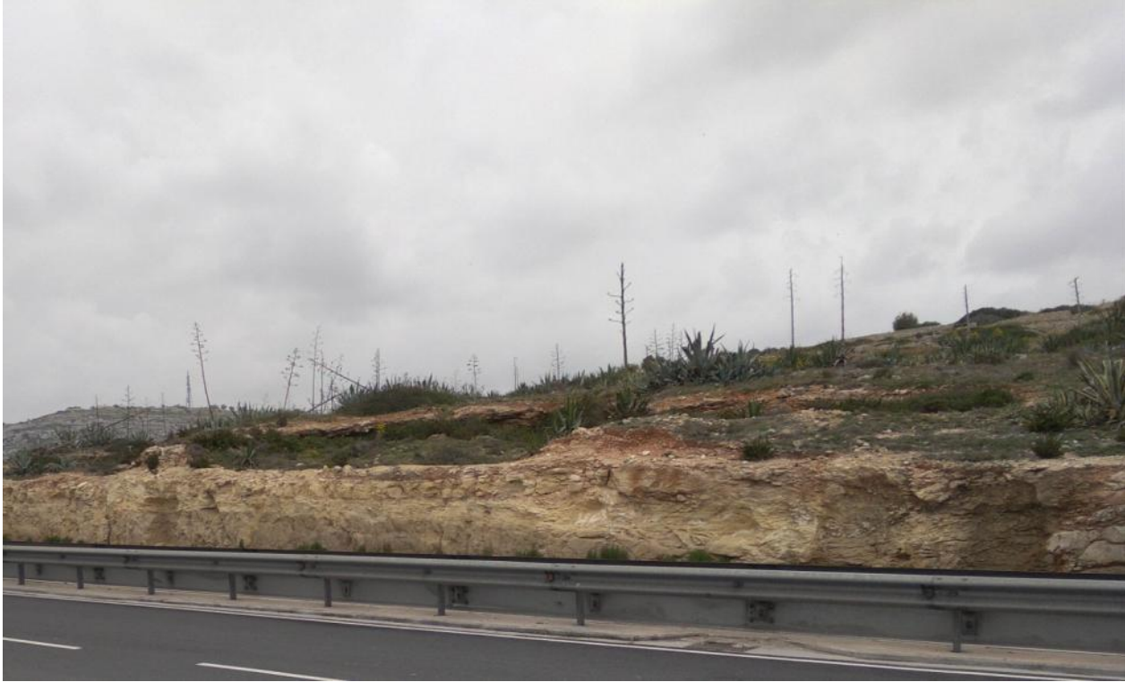
Figure 18: Photograph showing a surface lithified layer of red Quaternary slope deposits underlain by Lower Globigerina Limestone. Such deposits are usually associated with faults
