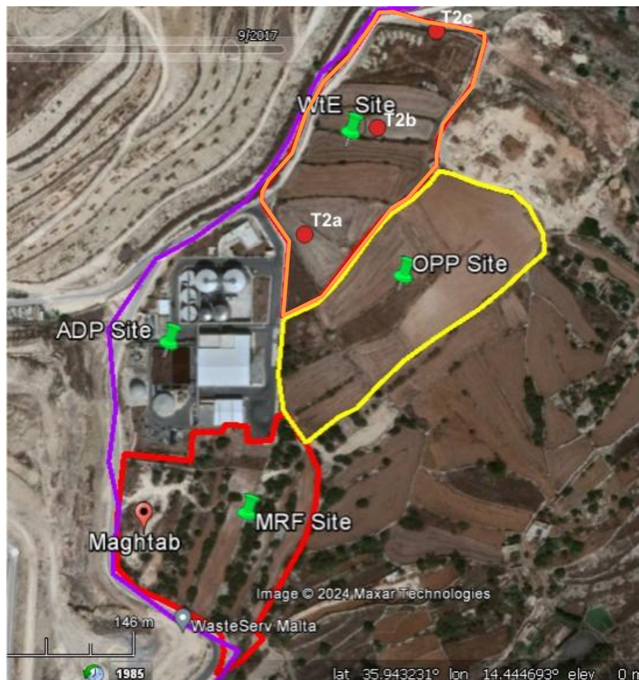
Figure 11: Plan showing the location of the boreholes drilled by continuous rock core sampling for the EIA for the WtE Facility.
