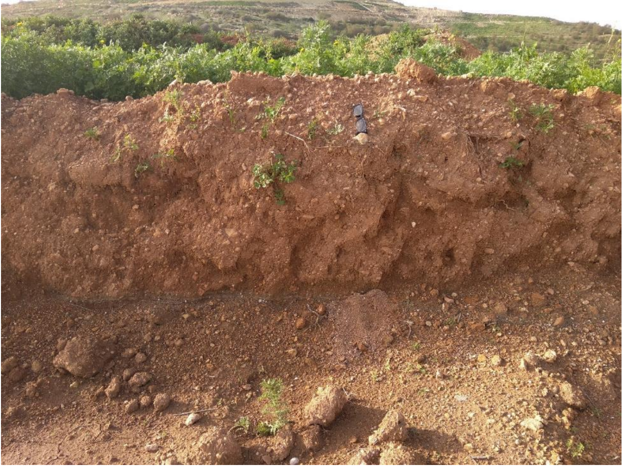
Figure 35: Photograph of a typical soil profile at the OPP site about 0.4m thick
