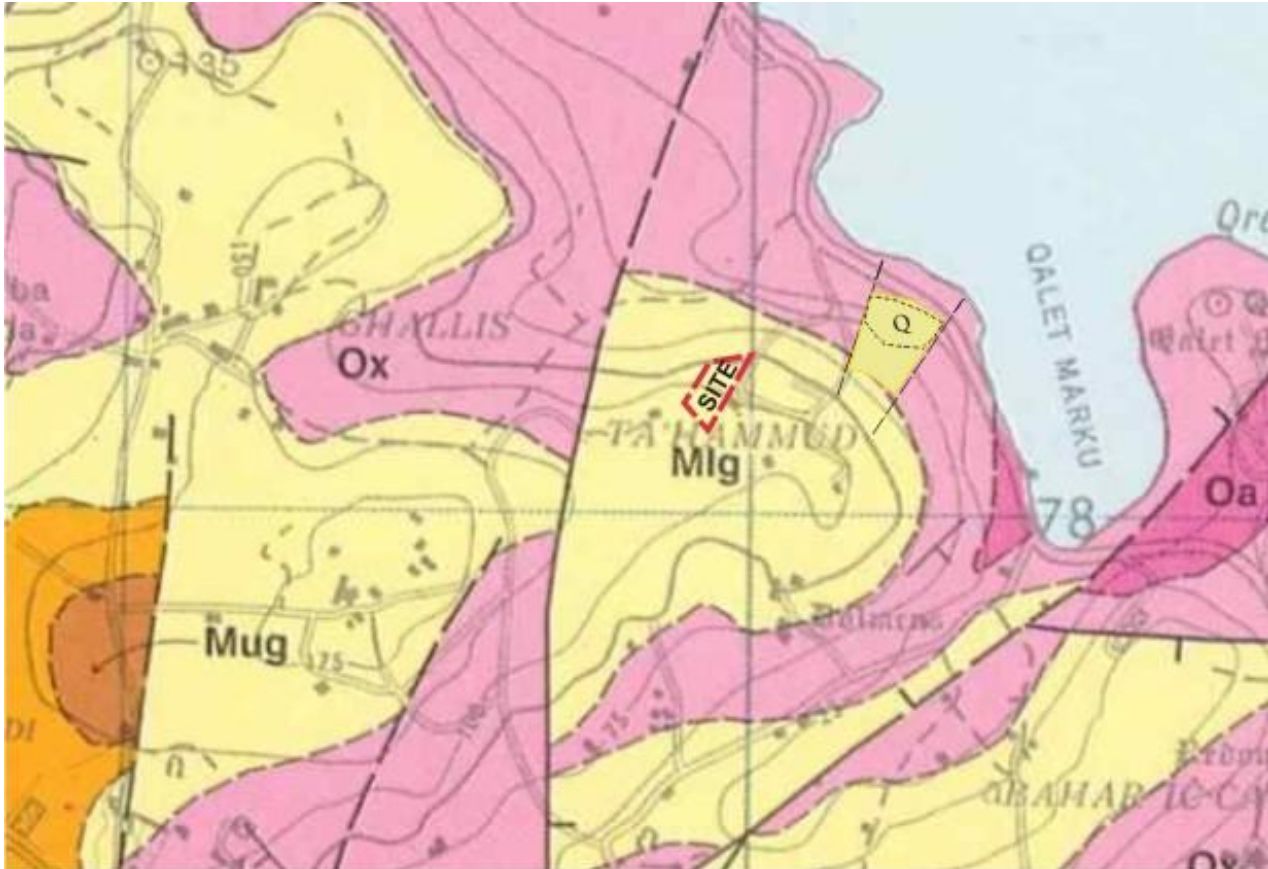
Figure 14: Geological map of Magtab and il-Ghallis (Modified after OED,1993) Q: Quaternary slope scree; Mlg: Lower Globigerina Limestone Mb; Ox: Lower Coralline Limestone Fm-Xlendi Mb Oa: Attard Mb
