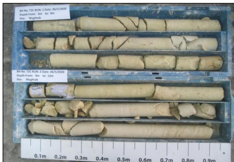
Figure 20: Photograph of Lower Globigerina Limestone core samples recovered from BHT2c Depth interval 6m to 12m below ground level
