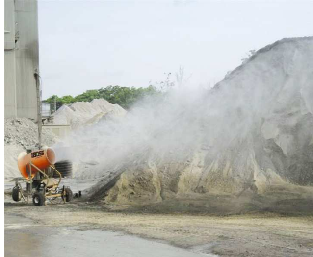
Example of a Water cannon wetting stockpiles
