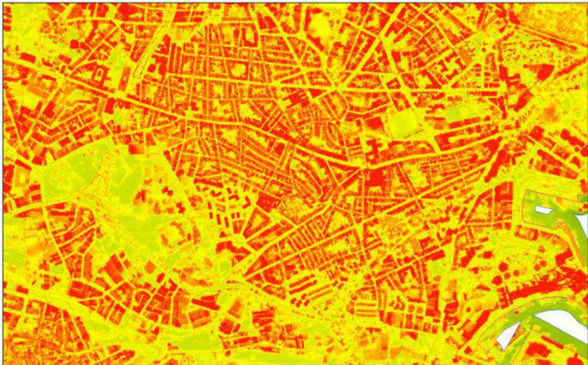
Figure 3-10. Sample of the relative height raster derived from DSM – DTM.
